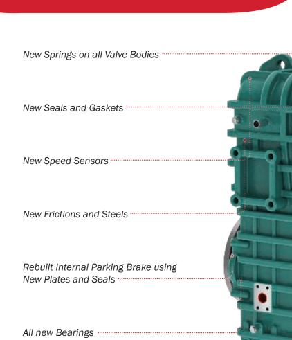
**100% Disassembly of the Transmission**
