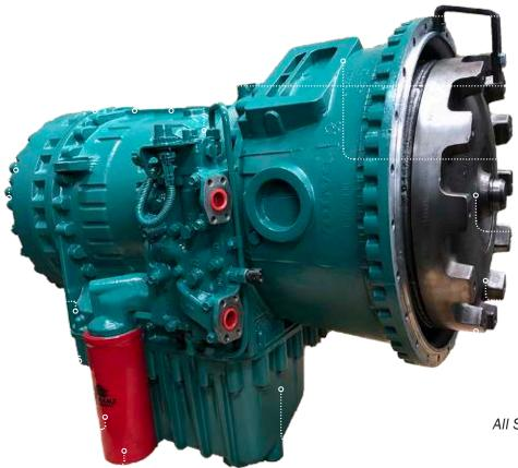
ALL Transmissions are Dyno Tested and undergo a 5-Step Evaluation: 1) Check Pressures. 2) Check to ensure No Leaks. 3) Check to ensure No Excessive Noise. 4) Function of Solenoid Valves are Evaluated. 5) Function of ALL Sensors are Tested using the TEM-CO TestBox.
